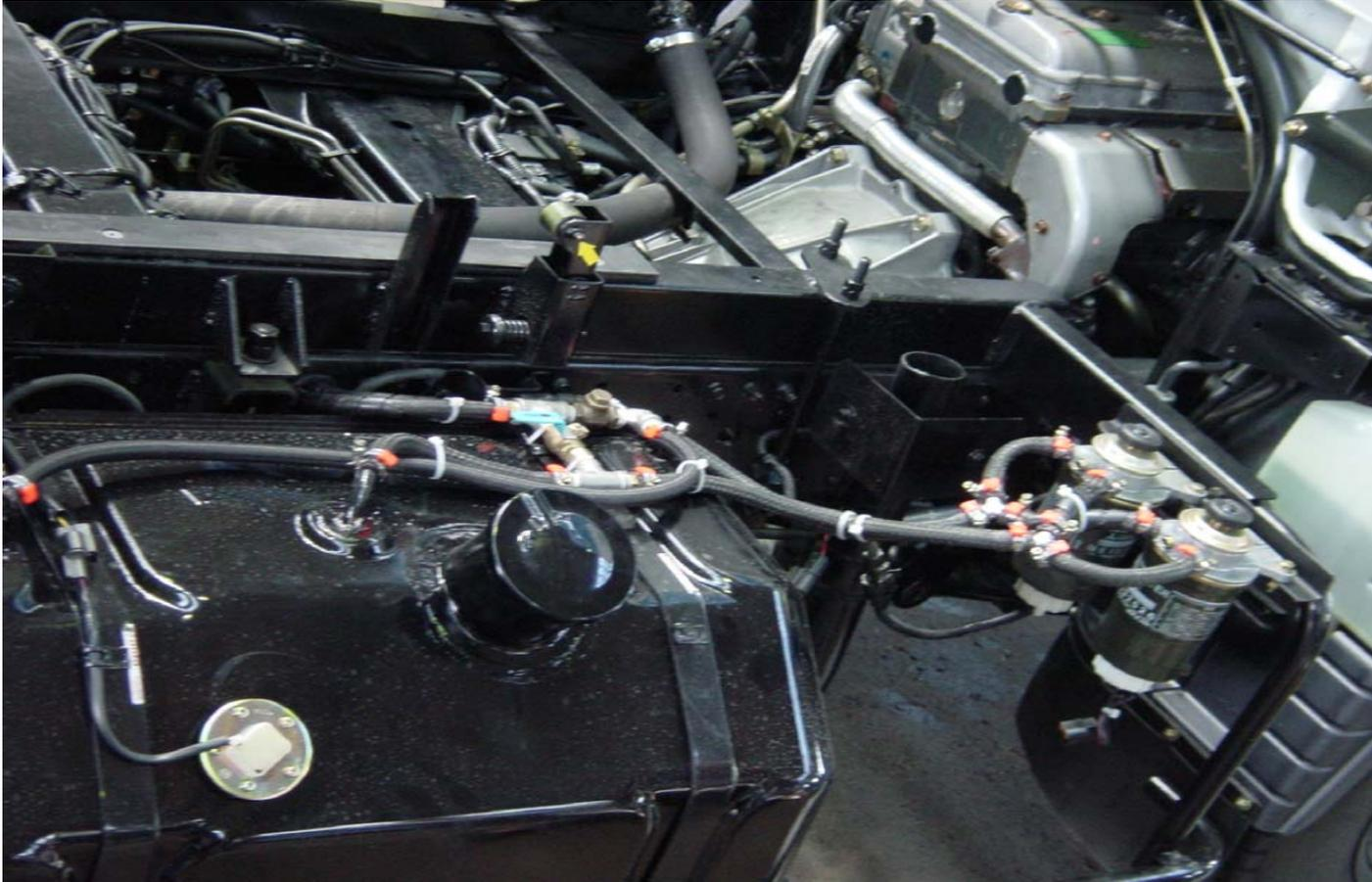
**Fuel hoses and packing ⇒ Alteration to string-slot rubber or fluorine rubber**
